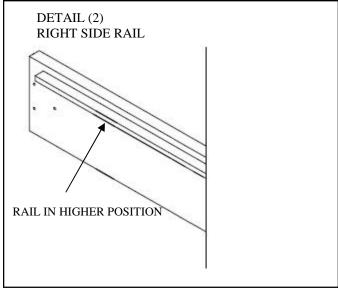
STEP 1: Attach the side rails (F) to the Headboard (E) by inserting the bolt heads at the end of the Side rails into the brackets on the Headboard. Push down to lock the bolts in place.
