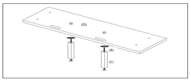
NOTE: The levelers at the bottom of the Support Legs (C) should be 3/4 unscrewed for hardwood floors and screwed all the way in for carpet.
